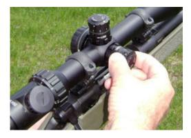
The most precise windage compensation results from target knobs, such as this 1/8th Minute-of-Angle knob on a Millett TRS scope. The Millett LRS has a <sup>1</sup>/<sub>4</sub> MOA knob.
