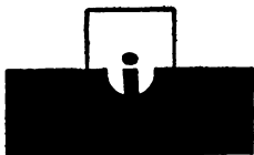
FIGURE 10. Correct Appearance of the Open and Peep Sights in Aiming.
